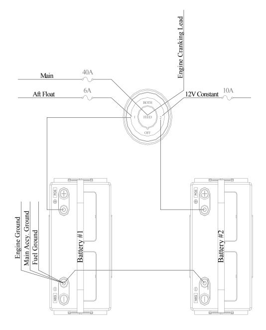
Battery Wiring with Select Switch
